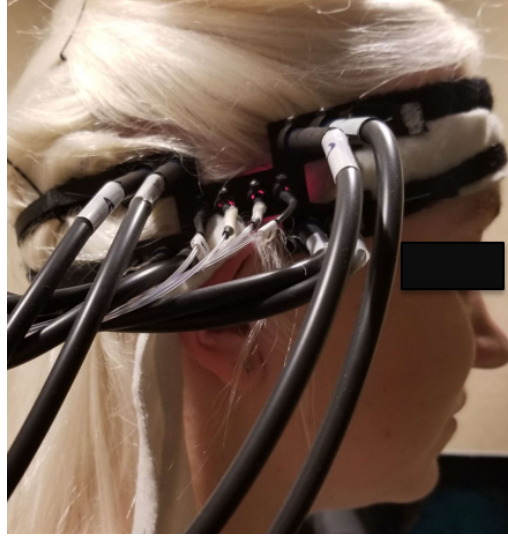
Figure 3.4: Placement of the probe on the T4 location above the Tragus on subject during an experiment
